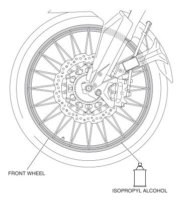
2. Remove the adhesive backing on the front wheel rim stripe as shown.
